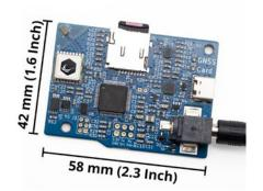
The battery-operated Datalogger STRATOmini measures and stores various data such as GPS coordinates, altitude and temperature, is extremely light at 13g and is the size of a matchbox.
